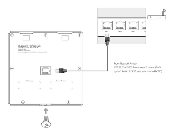
Slot-in Control Panel to the bracket, secure with screw and connect Ethernet cable (not supplied).
