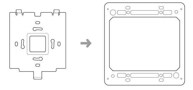
Use compatible screws to install bracket to an in-wall low voltage box (not supplied).
