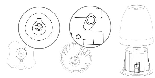
4 Install and fix hook screw with lock washer
